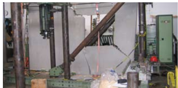
Testing of 12 m 2 large panels with window holes revealed in-plane shear strengths of up to 450 kN.
