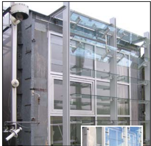
Fig. 1 The solar shading system with the lamellas in daylight redirecting position.
