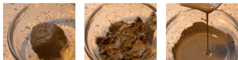
Example of a sensitive clay deposit which has a water content above the liquidation limit after thawing
