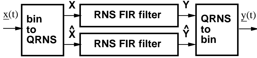
Figure 3.20: Structure of QRNS filter.
