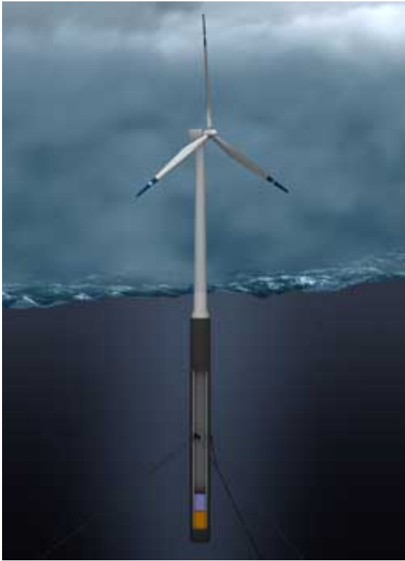
Figure 29: The floating wind turbine concept Hywind. Source: Norwegian Hydro and Solberg production.
