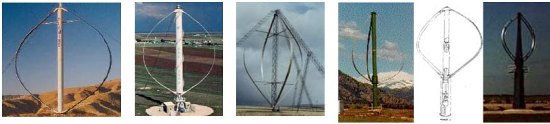
Figure 34: From left to right: Guy-wired (300 kW FloWind, 500 kW Sandia, 250 kW Chinook) and self-supporting (15 kW Tumac, 100 kW Fokker, Vestas tandem) Darrieus VAWTs
