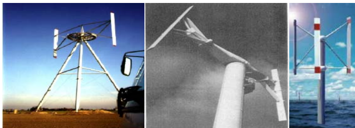
Figure 36: H-Rotors. Left-to-right: 300 kW Heidelberg rotor (MAGLEV generator), 500 kW VAWT, 3 MW UK LTD (concept study)
