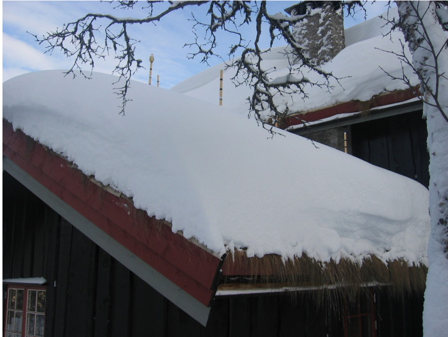
FIG. 3: Rule sticks for measurement of the snow depth on the roof of the cottage in Otta. Picture is taken the 21 st of January. Temperature sensor can be seen in top of the rule stick to the left.
