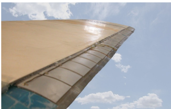
Figure 1.3: Variable airfoil geometry in wind turbine blade: deformable trailing edge geometry. The non linear deflection shape is obtained with piezoelectric laminae.
