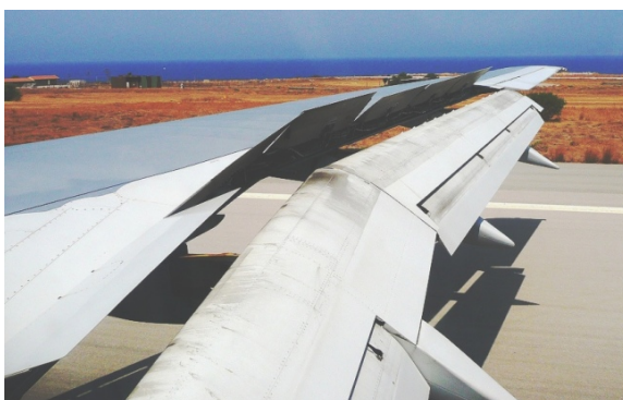
Figure 1.2: Variable airfoil geometry in aeronautics: flaps, aileron and deflectors on aircraft wing.
