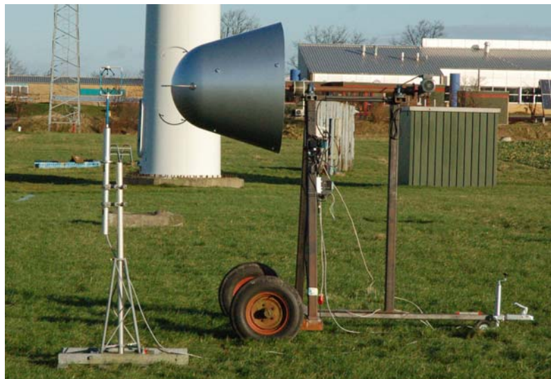
Figure 35 Arrangement of the S300 spinner anemometer with "new" sensors in comparison with the sonic anemometer at Risø test site
