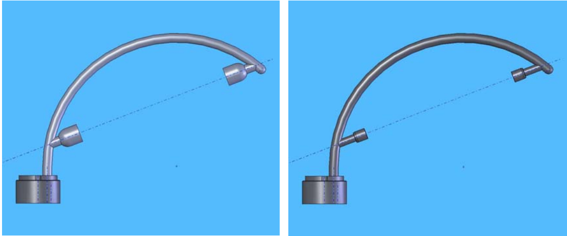
Figure 6 Prototype spinner anemometer sonic sensors specifically designed for the spinner anemometer. To the left with classic sensor heads. To the right with small sensor heads.
