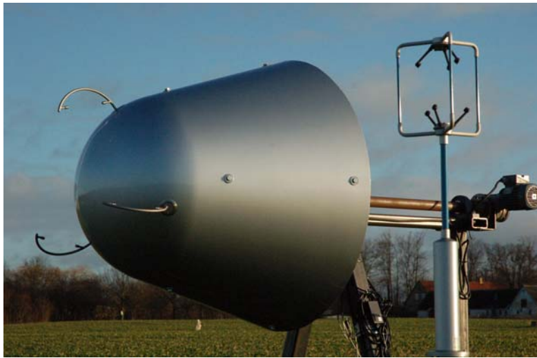
Figure 36 The S300 spinner anemometer and the Gill Windmaster in comparison
