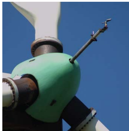
Figure 3 Arrangement of wind sensing instruments on a fixed arm extending from the spinner of a BOUNUS 55kW wind turbine
