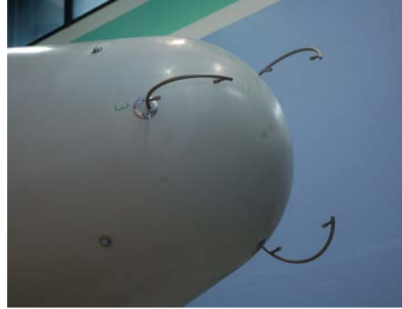
Figure 8 1D sonic wind sensors with small sensor heads, mounted from the inside of the spinner through the fittings on the 300kW wind turbine spinner. The sensor paths are tilted backwards in order for the wind to flow undisturbed into the paths. This eliminates flow distortion due to the sensor heads for the most important wind directions when the wind turbine is yawed into the wind.
