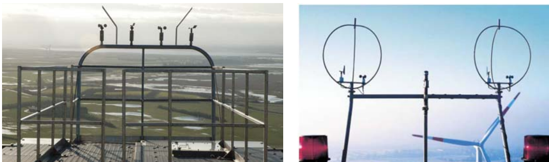
Figure 1 Arrangement of nacelle anemometry on top of the nacelle of modern wind turbines. The cup anemometers and wind vanes are mounted redundantly on support structures that may influence on the accuracy of the measurements of the instruments
