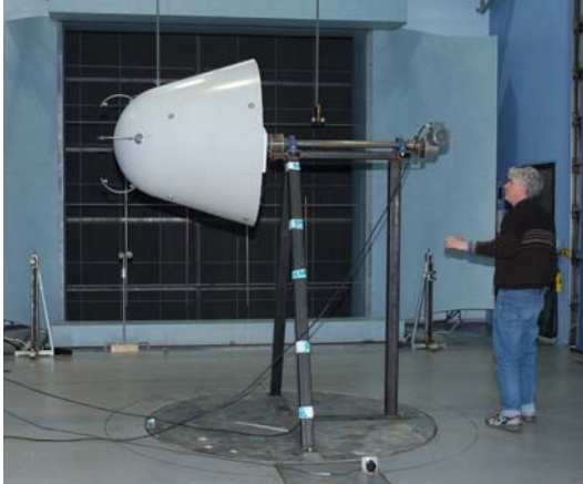
Figure 7 Arrangement for concept tests in a 4x4 m 2 wind tunnel. The spinner is seen yawed to -90° and the sonic sensors can be seen on the nose of the spinner. One sensor is horizontal in which position the sensor wind speed was measured with a sweep from -90° to 90° and related to the cup anemometer wind speed measured in the lower left corner of the inlet to the open test section.
