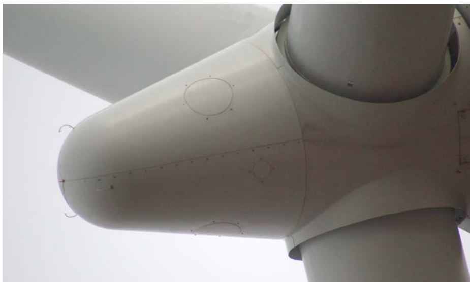
Figure 45 The three 1D sonic sensors mounted on the nose of the 3,6MW wind turbine spinner at the Risø DTU Høvsøre test site.
