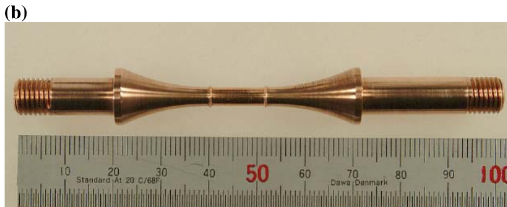
Figure 1. (a) Size and geometry of creep-fatigue specimens used in the out-of-reactor and in-reactor creep-fatigue tests and (b) a photograph of one of the creep-fatigue specimens used in these tests.
