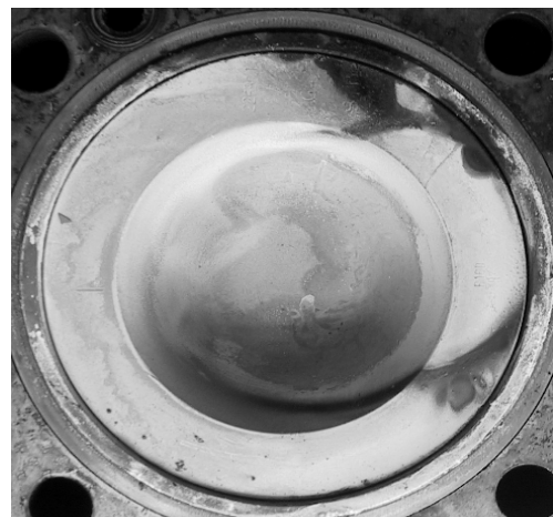
Figure 5: Top of cylinder after 1400 hours of operation.
