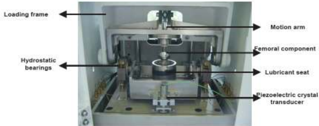
Figure 3.6. The friction measuring carriage and loading frame of the ProSim friction hip simulator.
