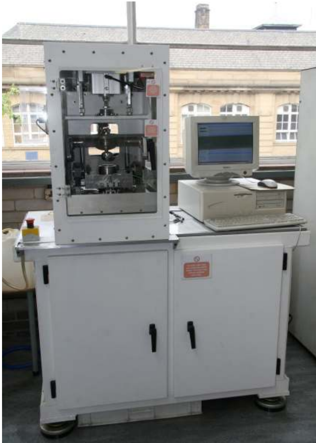
Figure 3.1. Picture of the Prosim Friction Hip Simulator used in this work for obtaining frictional torque and friction factor.
