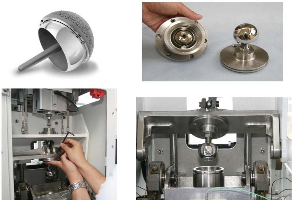
Figure 3.17. Assembling Metal head and cup on the Prosim Hip Friction simulator machine.
