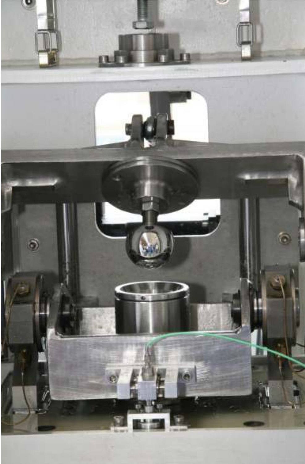
Figure 3.2.1. Friction hip simulator showing the fixed lower carriage with the cup holder and the moving carriage (rocker) with the femoral head.
