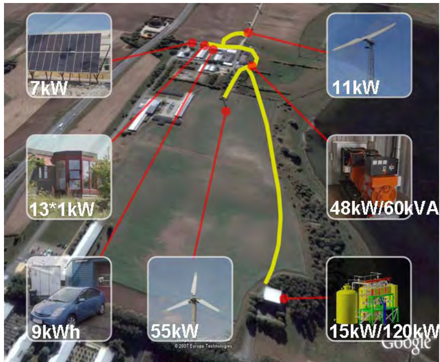
Figure 3 Outline of SYSLAB distributed energy systems test facility
