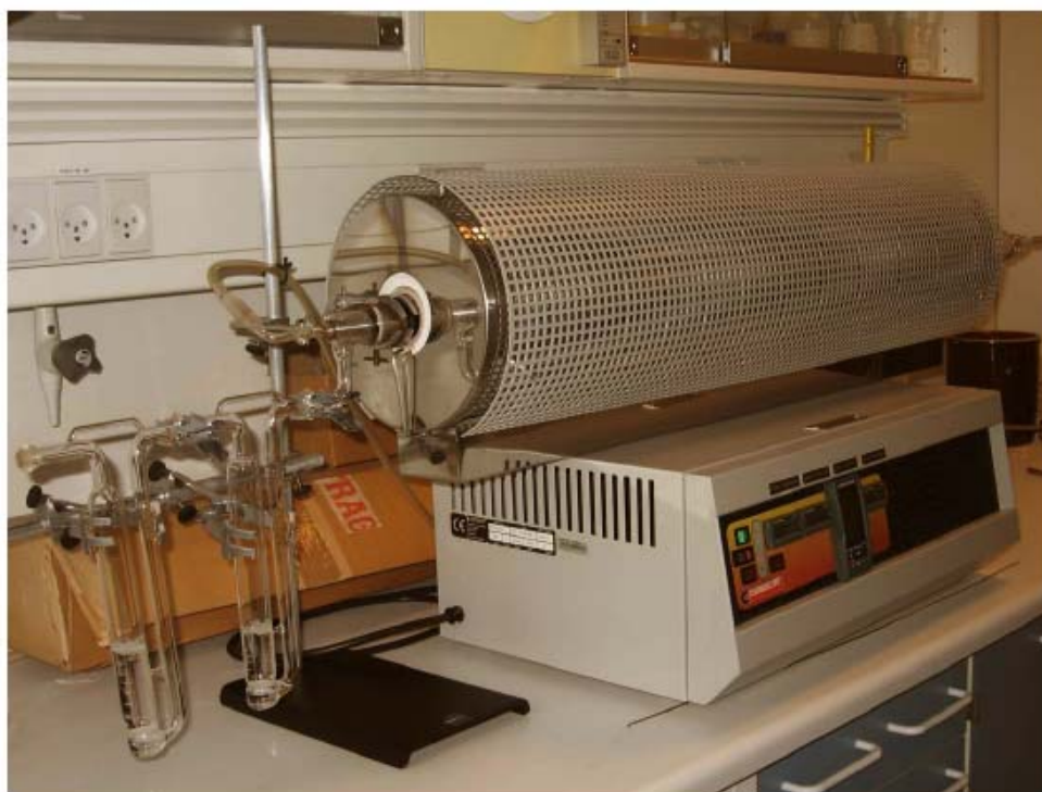
Fig. 4 Combustion equipment for the separation of iodine from solid samples
