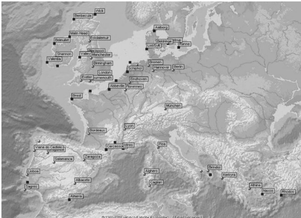
Figure 1. The meteorological sites used. The squares are stations of over 2000 full load hours. If the name is missing, it means that too many data were missing to use the station on its own
