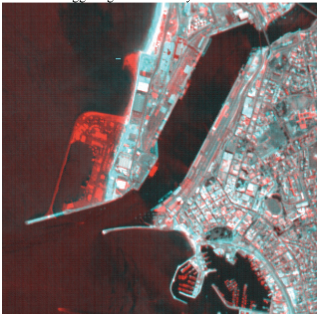
Figure 4. Image of week 46 showing the changes between 1986 and 2004: new harbour (red) but also coastal erosion (cyan) at Fremantle/Perth, copyright SPOT and ESA
