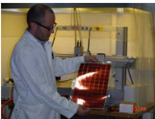
A picture of the first 0.1 square metre plastic solar cell made by screen printing at Risø on the 01. December 2004.
