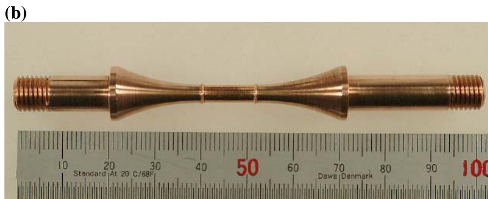
Figure 1. (a) Size and geometry of the creep-fatigue specimens used in the out-of-reactor and in-reactor creep-fatigue tests and (b) a photograph of one of the creep-fatigue specimens used in these tests.
