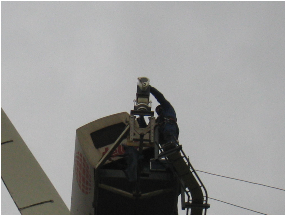
Figure 3-1 The QinetiQ ZephIR lidar head mounted on the downwind end of the Tellus nacelle. From [15].
