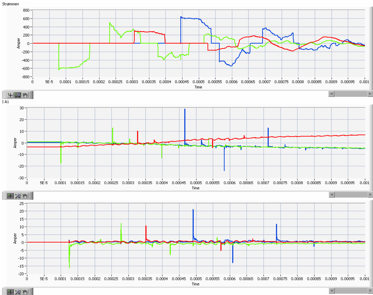
Figure 8 Current measurements at three locations during closing of the line breaker. Top: Transform platform, Middle: Turbine A01, Bottom: Turbine A09. Time: 50µs/div.
