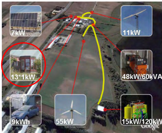
Figure 2. Components in SYSLAB
