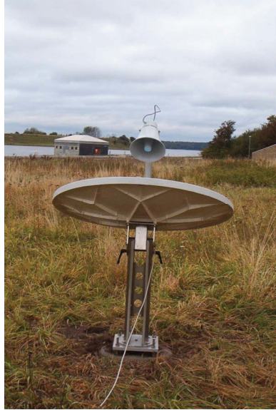
Figure 16. The Heimdall sodar transmitter at Risø. The speaker is located in the focus of the antenna disk.
