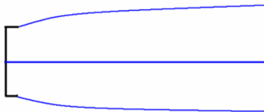
Figure 5-2 Geometry used in the actuator cap/vortex tube model. Black: actuator cap. Blue: distinct root vortex and tip vortex tube.
