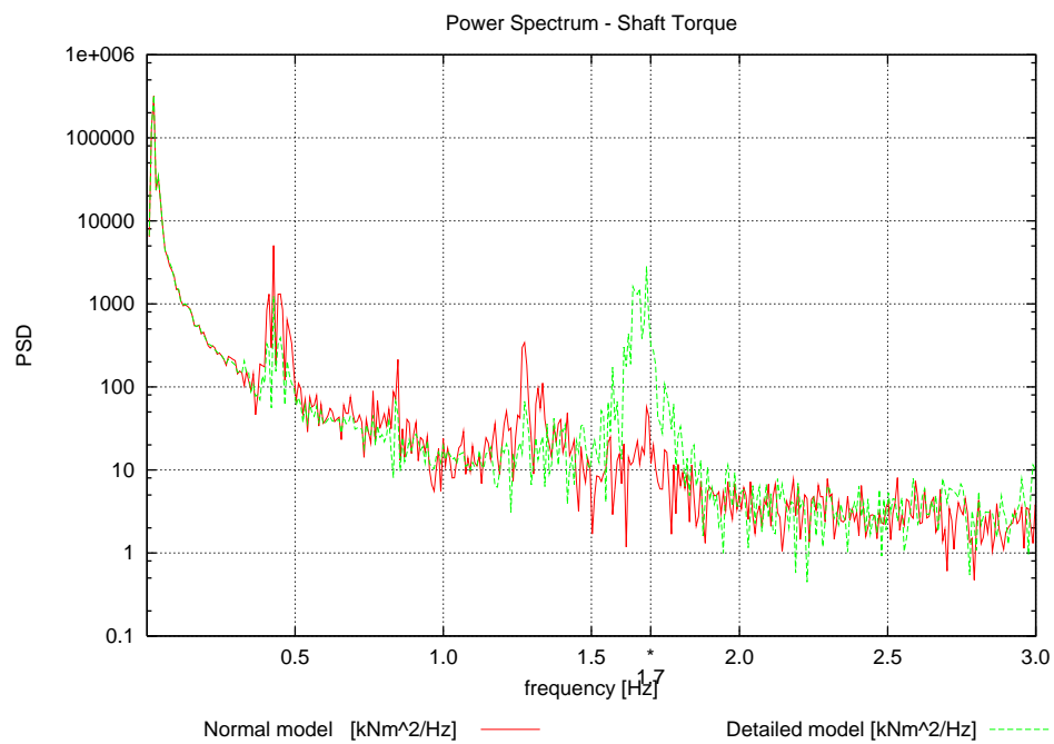
Figure 9-3: Comparison between shaft torque for normal and detailed aeroelastic model.
