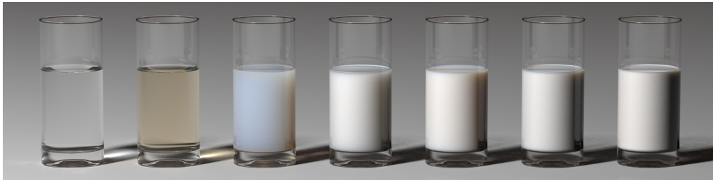
Figure 1: From the paper by Frisvad et al. [6]: Rendered images of the components in milk as well as mixed concentrations. The scattering properties of the components and the milk have been computed using a new scheme for robust evaluation of the Lorenz-Mie coefficients when the host medium is absorbing. From left to right the glasses contain: Pure water, the host medium (water and dissolved vitamin B2), water and protein, water and fat, skimmed milk, regular milk, and whole milk.
