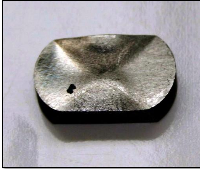
Fig 7. Photograph of diametrically compressed disc of Fe-1.4C-0.6Si-0.85Mo when the plastic zones emanating from the platen contact regions meet at the disc centre. The height of the disc, warm forged at 700°C at a strain rate of 10^{-3} \text{ s}^{-1} , reduced from 13.5 to 9.2 mm.
