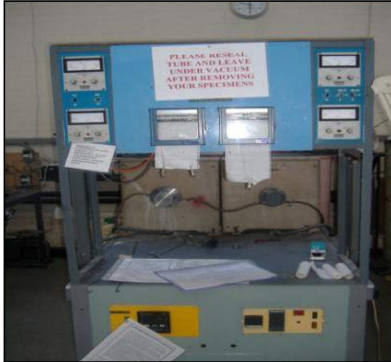
Figure.3.6: Laboratory vacuum sintering furnace.
