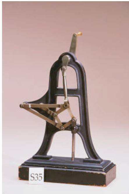
Fig. 4 Peaucellier straight-line mechanism (credit line: Jon Reis/www.jonreis.com)
