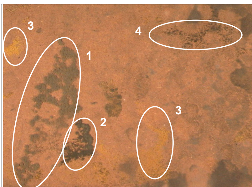
Figure 27. A MDF plate (20×14 cm) from paper 10, after 4 months at 95%RH and 10°C. # 1 and 2 are P. chrysogenum growth (2 mm high) and #3 is a Eurotium Sp., #4 is Ulocladium sp., and the rest of the material is partly covered with a mixture of A. versicolor and P. chrysogenum .
