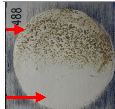
Figure 9. The influence of too high air velocity on A. versicolor growth in one side of the set-up.
