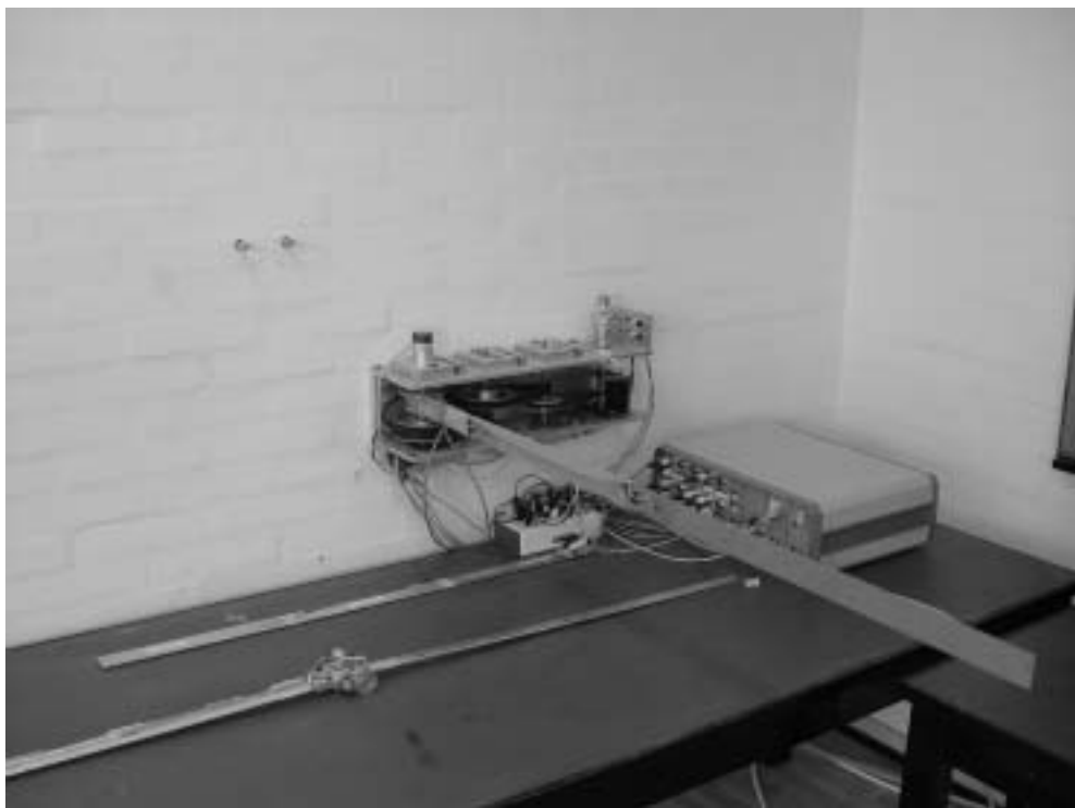
Figure 19.1: The robot consists of hub where different type of arms can be mounted. Notice the wall mount enabling the robot to move in the vertical plane instead of horizontally. The arm mounted is a 1DOF arm; on the table are another 1DOF arm and an arm with two flexible links. It is equipped with tachometers and strain gauges in order to measure the link angles and deflection, respectively.
