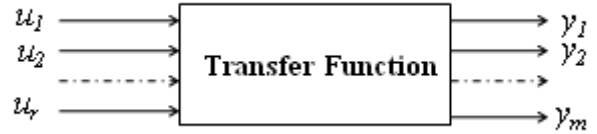
Figure 1 A multivariable technique: a system with r inputs and m outputs
