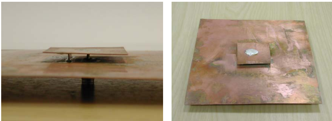
Figure 6.46 Prototype harmonic rejection antenna with partially shorted, side view (left) and top view (right).
