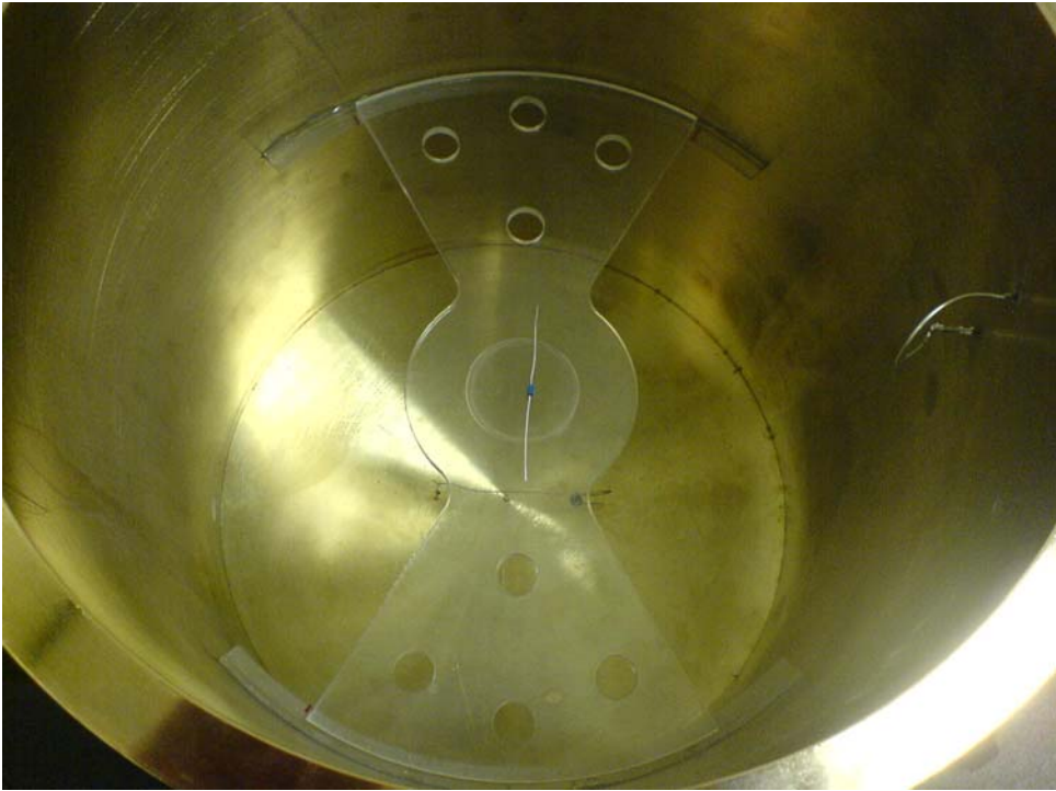
Figure 6.32: Orientation of the diode orthogonal to the transmitted antenna
