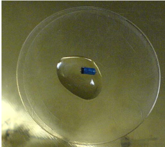
Figure 6.34: UHF diode without leads and loaded with 60 \mu l water
