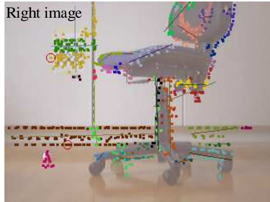
Fig. 4. The resulting clusters after filtering is shown on top of one of the original images. In total 848 3D detections are shown in 36 clusters.
