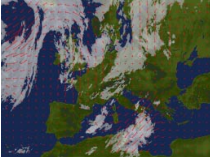
Fig. 3: The clouds have been segmented using the technique described in Section A and the corresponding estimated flow field is overlaid as red vectors. The starting point is marked with a dot and the length is proportional to the speed.
