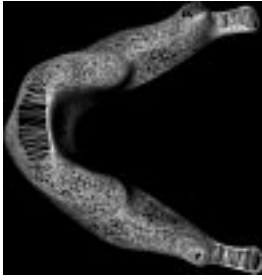
Figure 11. The deformation vectors are moved too far away from the surface (The value of \sigma is too high) resulting in a wrong projection back onto the surface. The resulting field is torn apart in the high curvature regions near the condyles and the teeth. See also text in Section 5.2.
