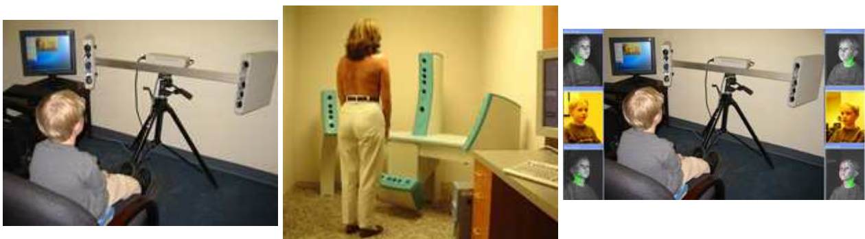
Figure 1: Minolta VIVID 910 3D laser/camera scanner ( www.minolta.com ) and scanned face
