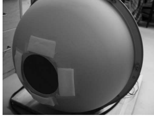
Fig. 1. Integrating sphere with optimal illumination conditions used to capture the images.
