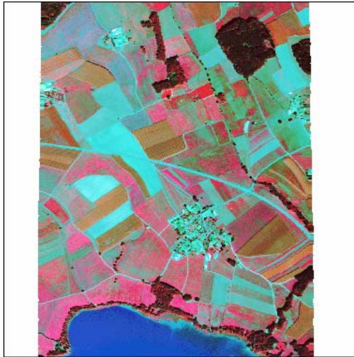
Figure 2: HyMap data from 4 August 2003 at 10:23 UTC 798 nm (red), 677 nm (green), 570 nm (blue)
