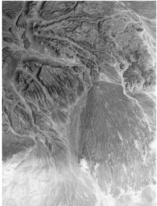
Fig. 9. Mosaic of two Landsat ETM+ scenes from May 2 and May 27, 2000 without radiometric normalization.
