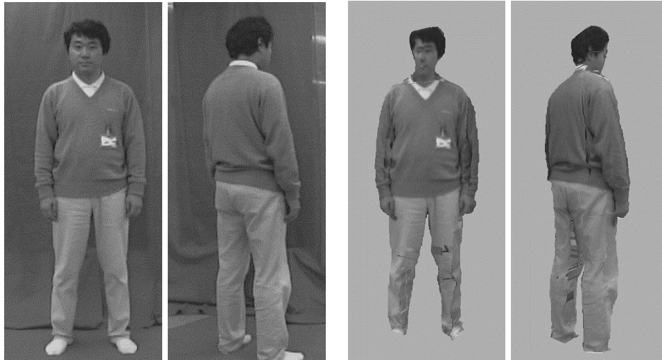
Figure 12: Human being modelled using perspective algorithm. 3D model creation took 19 minutes on a SiliconGraphics IRIS 4D/420VGX using 8 views with an average of 261 occluding contour polygon arcs in each view image. Left 2 images show original. Right 2 images show model with texture.
