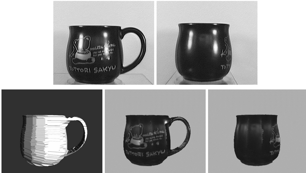
Figure 10: Cup modelled using perspective algorithm. 3D model creation took 23 minutes on a SiliconGraphics IRIS 4D/420VGX using 12 views with an average of 170 occluding contour polygon arcs in each view image. Upper row shows original. Bottom row shows model with and without texture.
