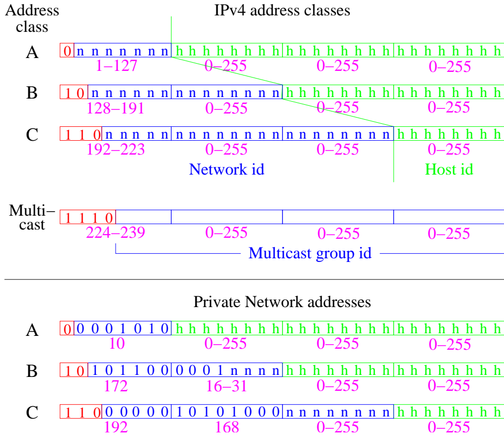
Figure 6.3: IPv4 addresses (above) and Private Network addresses (below)
