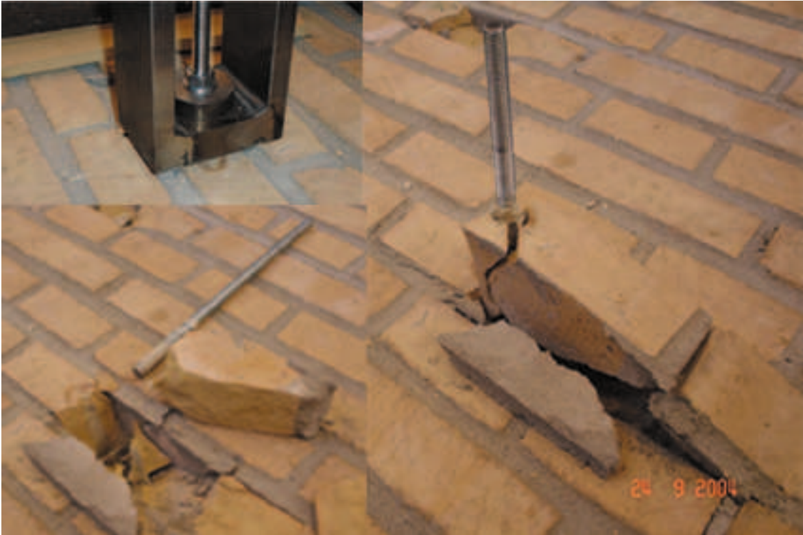
Figure A.3: The failure mode observed
