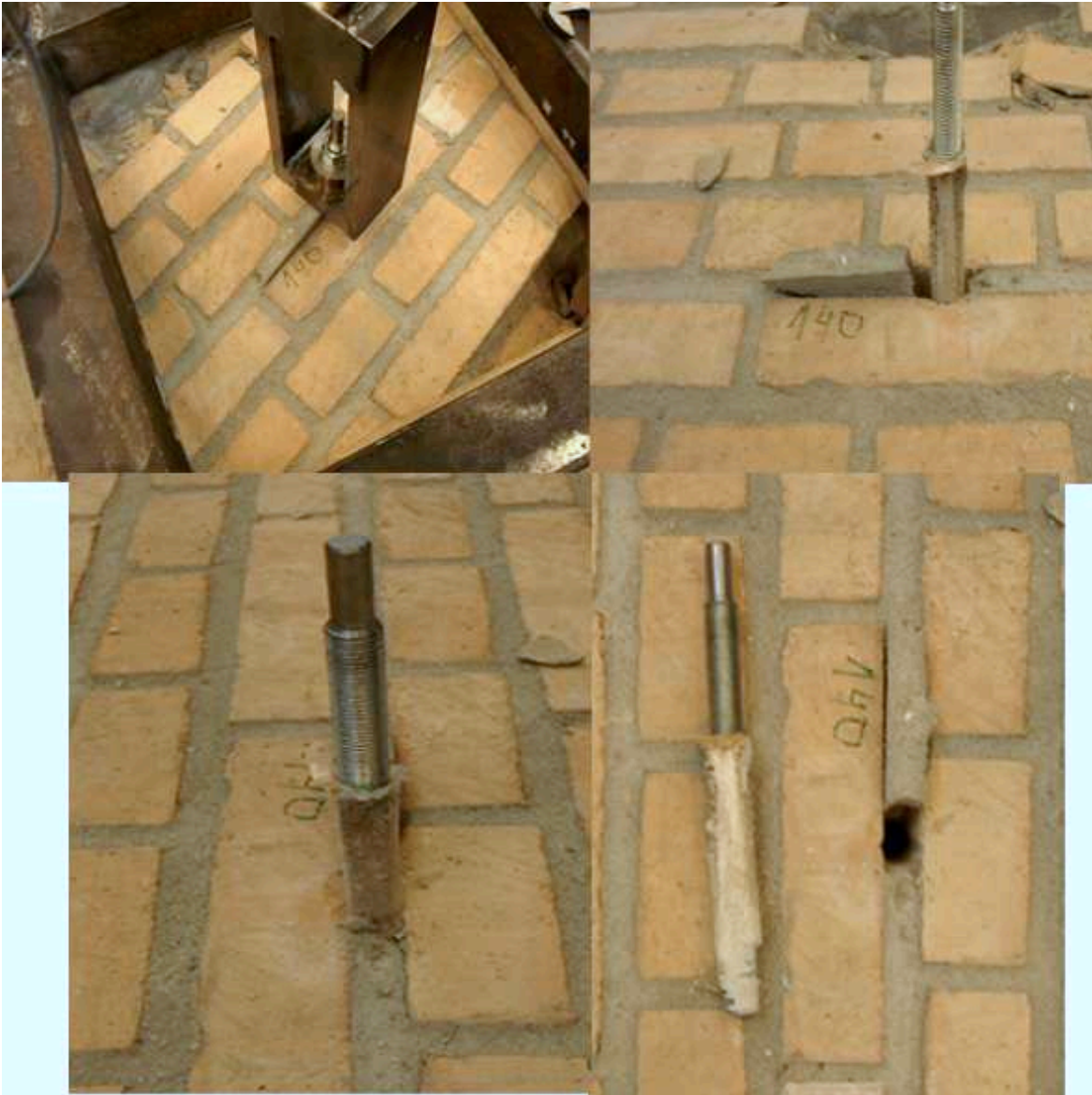
Figure A.105: The failure mode observed
