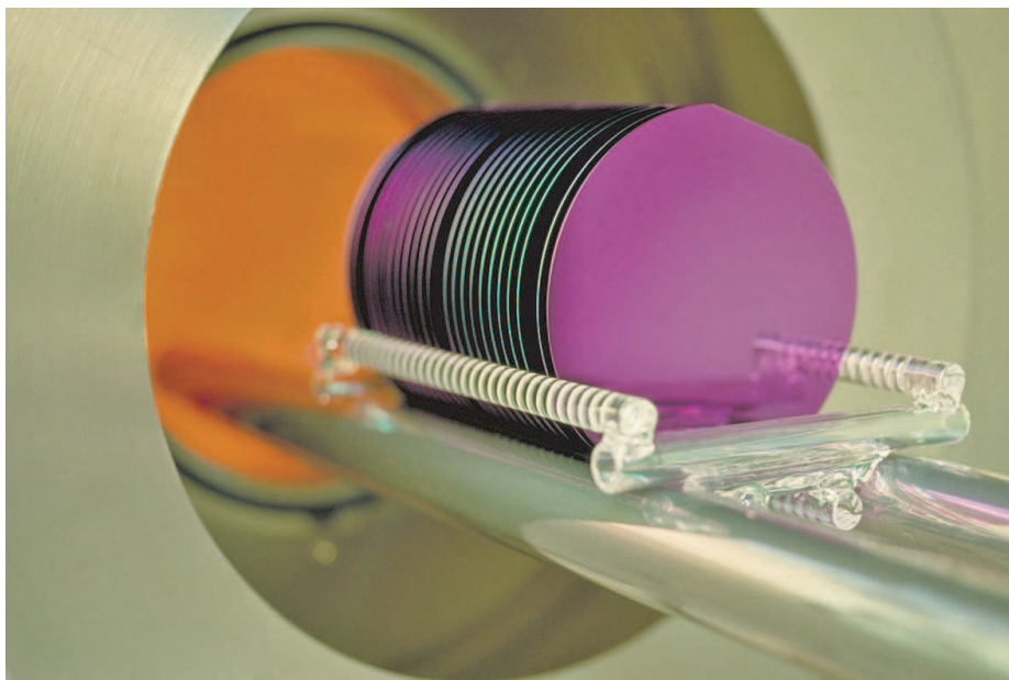
Figure 4.3: Silicon wafers being transferred into an anneal oven. The wafers are usually backed in the oven for 4 hours. The temperature and the atmosphere are controllable. Picture is made available by the COM photographer Lasse Rusborg.
