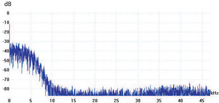
Figure 3.6: Fourier transform of the phase noise signal measured. The noise floor of the used oscilloscope is -80dB. The noise is severe up to 5 kHz and it has measurable frequency components up to 10 kHz.
