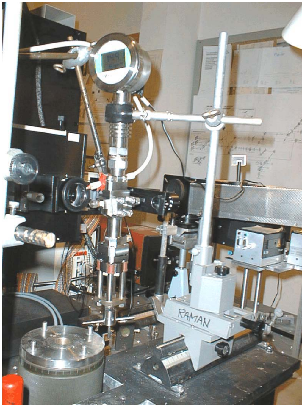
Fig. 2.8. Photograph showing the titanium cell, ready for Raman measurements. The pressure is read on the transmitter to 149 bar R (14.9 MPa R ). The little red lamp just in front of the entrance to the spectrometer is a Neon lamp. If a spectrum of a sample is obtained simultaneously with lines from this Neon lamp it is possible to accurately calibrate the spectrum with respect to wavenumber position, as will be discussed in Chap. 5. Photo: S. Helmark.
