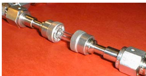
Fig. 2.2. Photograph showing the quartz tube inserted in the tube connectors (Cajon ultra torr adapter). Photo: S. Helmark.
