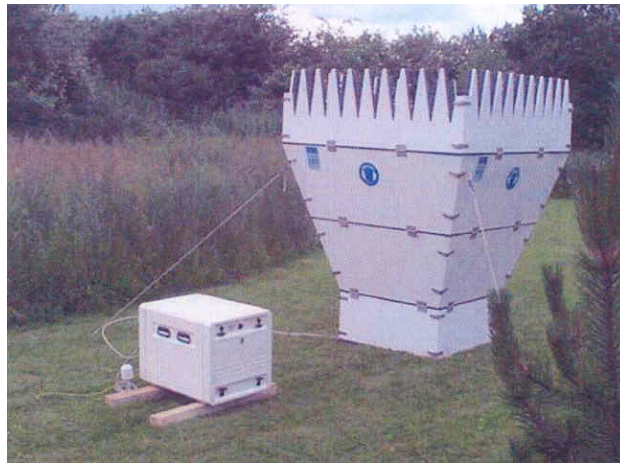
Figure 1: METEK Doppler PCS-2000/24 low power version SODAR.
