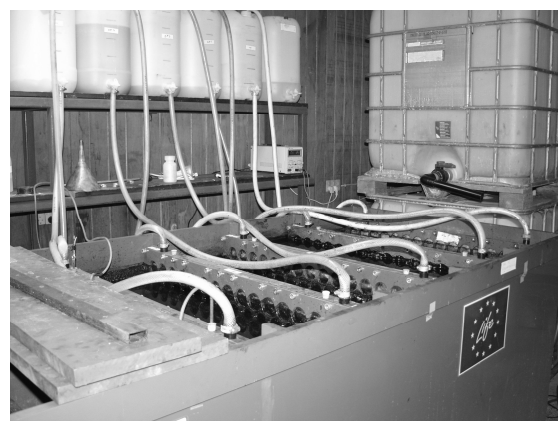
Figure 4: The pilot plant for electrodialytic remediation. In the present experiment, the distance between the electrodes is approximately 140 cm. For each 35 cm, a concentration compartment has been inserted, thus dividing the plant into 4 separate desalination compartments containing app. 300 L ash suspension each.
