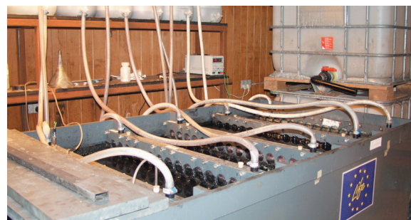
Figure 3: Pilot-scale remediation experiment. The distance between the electrode units is approximately 140 cm. For each 35 cm, a "concentration compartment" has been inserted, thus dividing the plant into 4 separate desalination compartments (ash compartments). Each desalination compartment contains app. 300 L of ash suspension.
