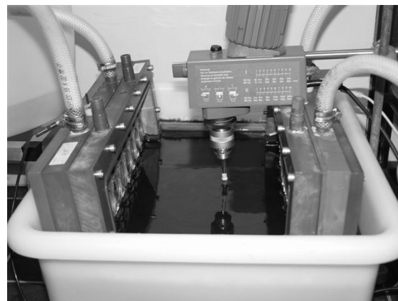
Figure 3: 25 L bench scale experiment. The distance between the two electrode units is approximately 30 cm.
