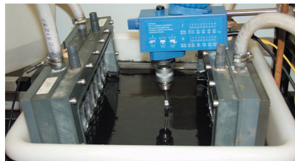
Figure 2: Bench-scale electro-dialytic remediation experiment containing 25 L fly ash suspension. The electrode compartments are separate units, submerged in the fly ash suspension to be remediated. The distance between the electrode units is approximately 30 cm.
