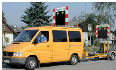
Figure 3: Traditional ‘falling weight’ deflectometer equipment.
