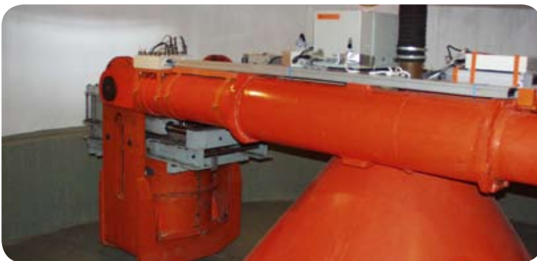
Beam centrifuge at BYG•DTU
