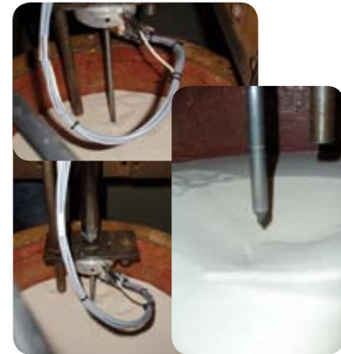
Pictures from test in centrifuge with small scale Cone Penetrometer.
