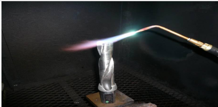
Figure 6.11 (c): The heat Treatment part been heated
