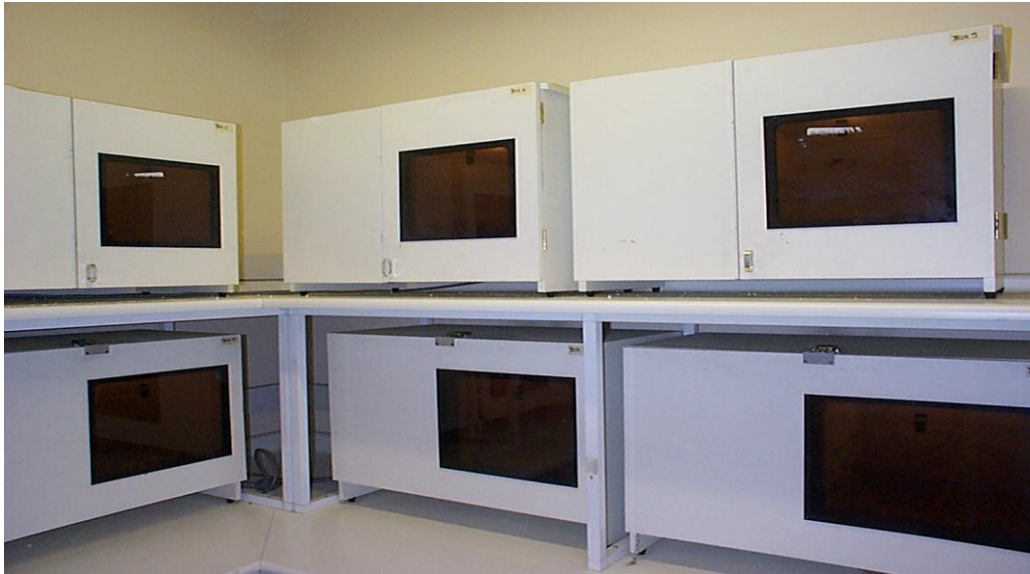
Figure 3.2.2a Identical Skinner boxes in test room.
