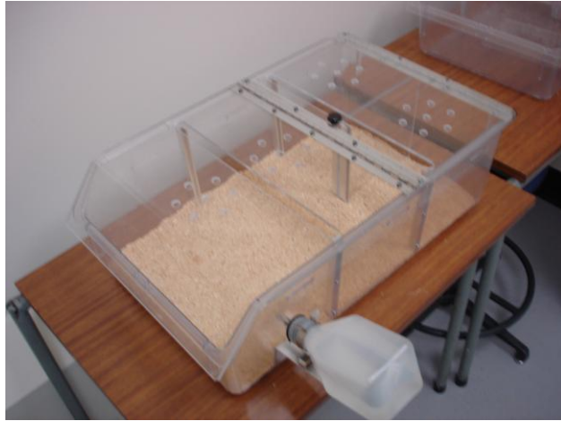
Figure 2.2.3a: Photograph of the attentional set-shifting test box, plexiglas dividers were inserted into the visible slots in the lid.
