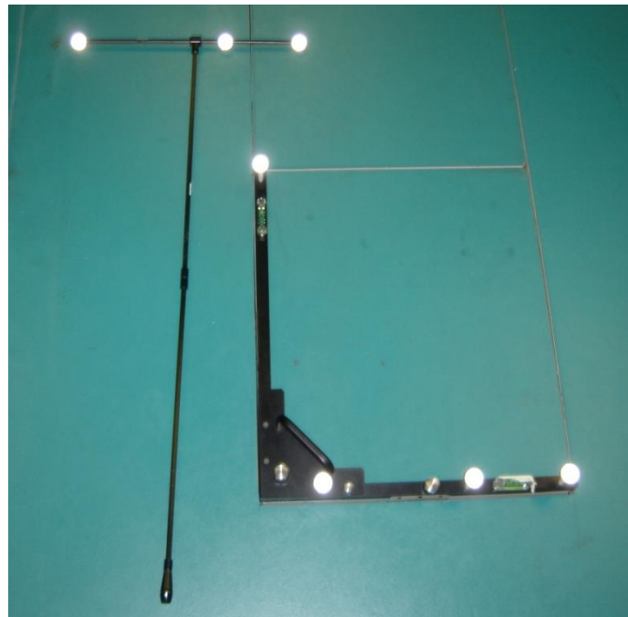
Figure 3.10. The L-Frame placed at the origin of the capture volume and the 'T' shaped wand used for static and dynamic calibration respectively.
