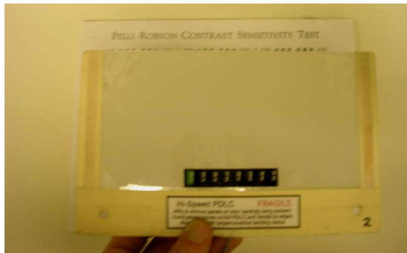
Figure 3.8. LCD sheet in the a) transparent condition and b) opaque condition which eliminates all visual information.
