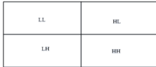
Figure 2-3 The result of 2-D DWT decomposition.
