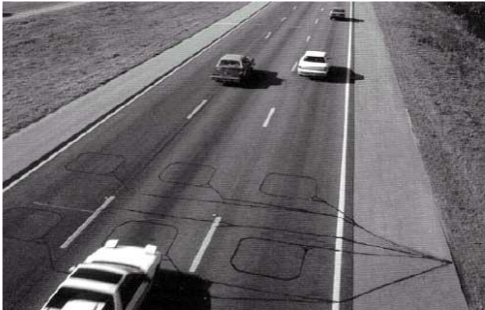
Figure 2.1: Inductive Loop Detector System[92].
