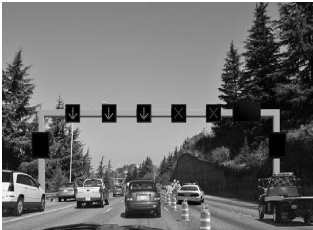
Figure 2.7: Green arrows and red crosses on VSL show which lanes are open and which are closed [178].
